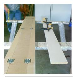
A simple jig is fabricated that makes bending of the screen easy.
